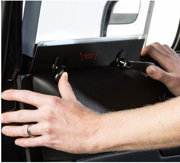
▲ Figure 15. Flipping the bracket handles outward to lock
