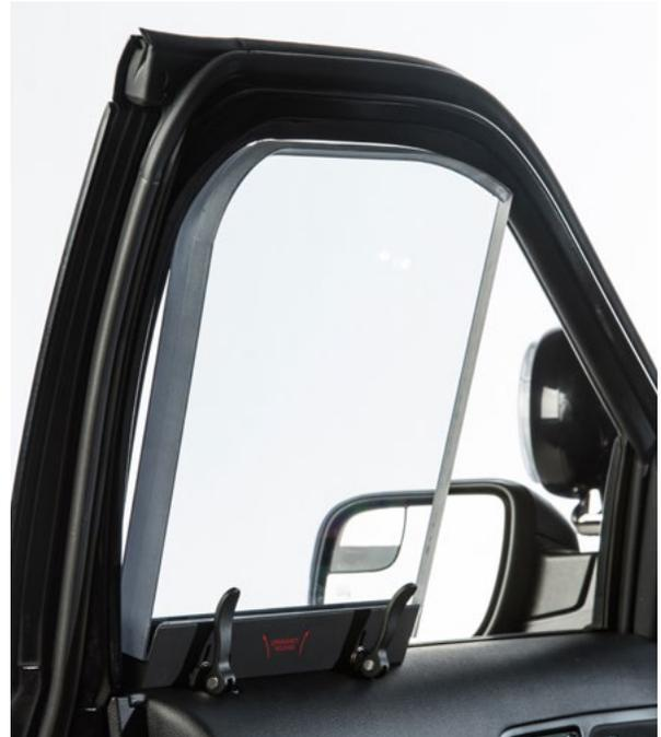
▲ Figure 11. Groove along top of armor is aligned with weatherstrip along top of window frame
