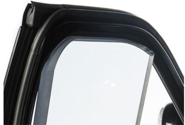
▲ Figure 13. Weatherstrip is seated in armor groove uniformly
