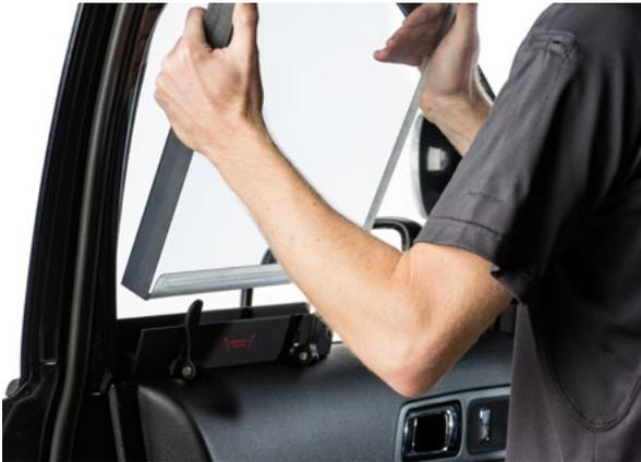
▲ Figure 9. Placing the window armor into the bracket
