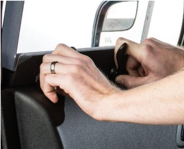
▲ Figure 12. Rotating the bracket handles inward
