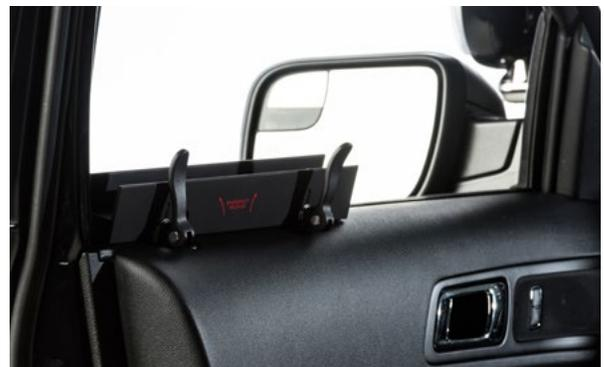
▲ Figure 8. Bracket door lock post cutout is aligned with the door lock post
