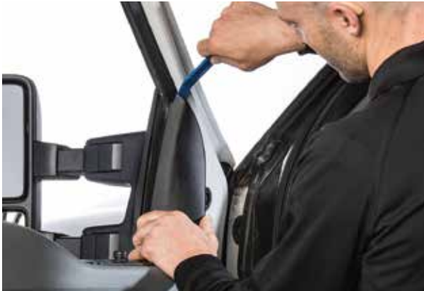
▲ Figure 19. Removing the side-view mirror mounting cover
