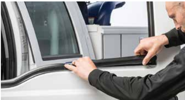
▲ Figure 26. Pressing down the window weatherstrip
