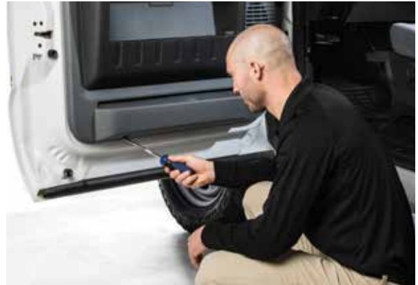
▲ Figure 9. Removing door compartment screws
