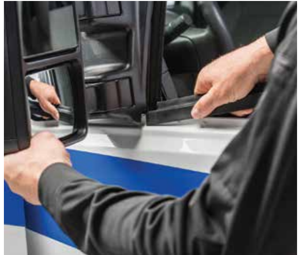
▲ Figure 21. Removing the window weatherstrip
