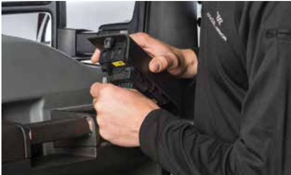
▲ Figure 12. Disconnecting the wiring harnesses
