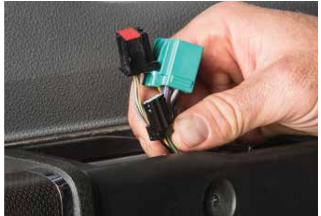
▲ Figure 18. Ensuring the wiring harnesses are visible
