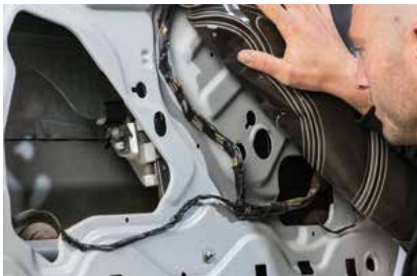
▲ Figure 15. Removing the regulator bolts
