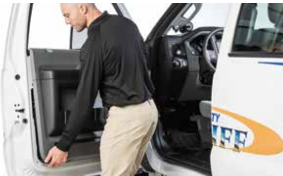
▲ Figure 13. Pulling the door panel up and away from the door
