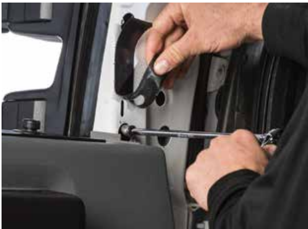
▲ Figure 20. Loosening the side-view mirror nuts
