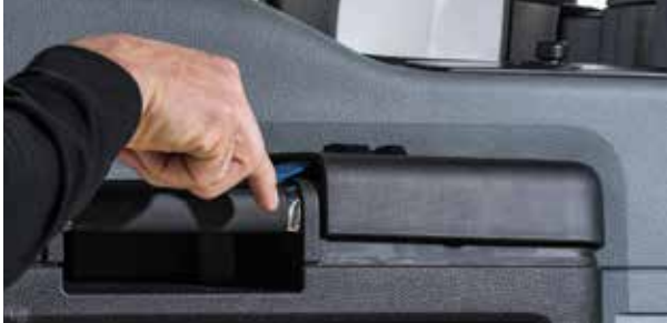
▲ Figure 11. Removing the window control panel
