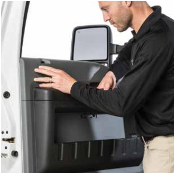
▲ Figure 17. Aligning the door lock pin and snapping the upper edge of the door panel on the interior
