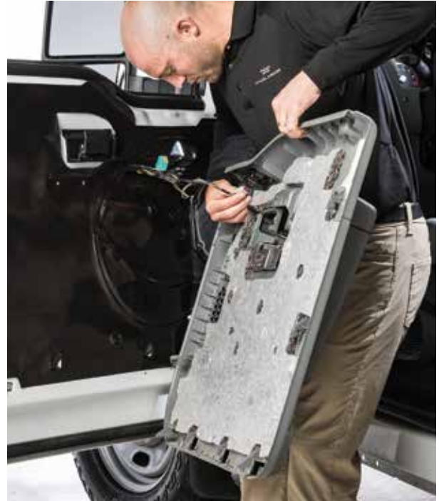
▲ Figure 14. Disconnecting the wiring harnesses
