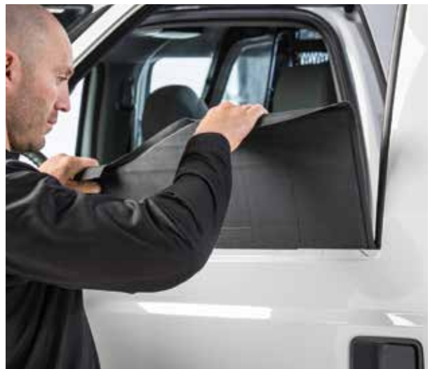
▲ Figure 23. Inserting the Ballistic Door Panel into the door
