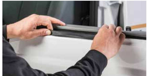
▲ Figure 25. Positioning the nylon folds over the window frame
