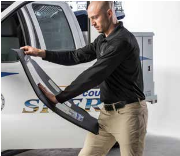
▲ Figure 22. Bending the bottom of the panel away from you
