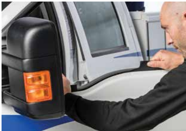
▲ Figure 24. Positioning the Ballistic Door Panel
