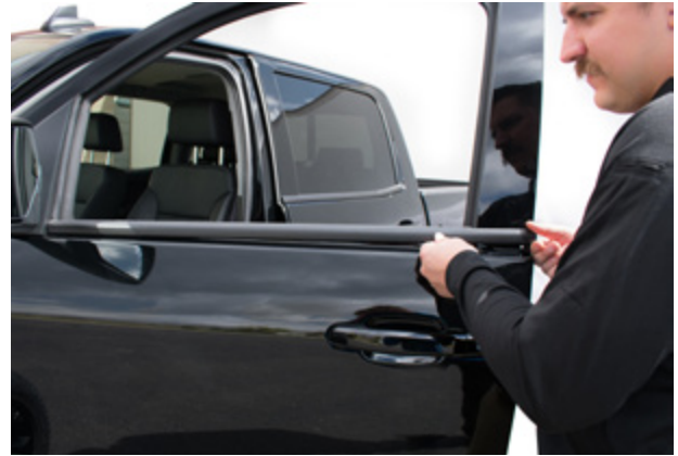
▲ Figure 9. Removing outer window weatherstrip
