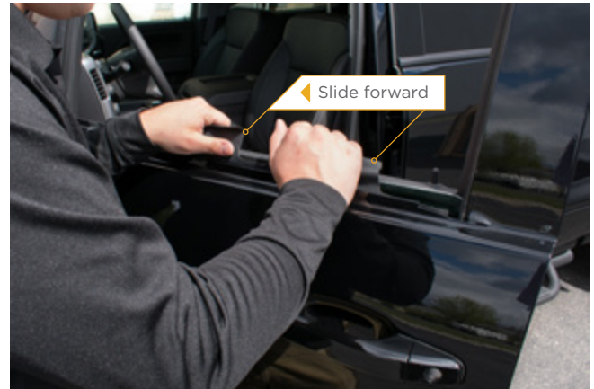
▲ Figure 12. Gripping and sliding the ballistic door panel forward into place
