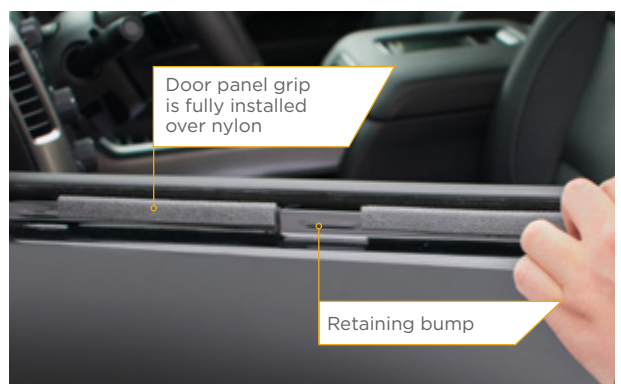
▲ Figure 15. Final placement of door panel grips.
