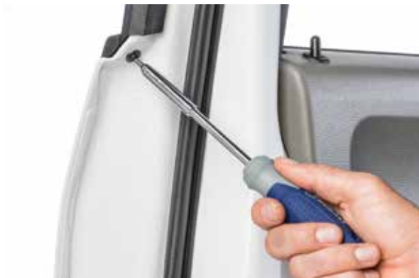
▲ Figure 14. Replacing outer window weatherstrip screw
