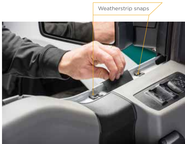
▲ Figure 12. Proper alignment of nylon fold with window frame
