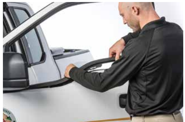
▲ Figure 8. Removing the outer window weatherstrip
