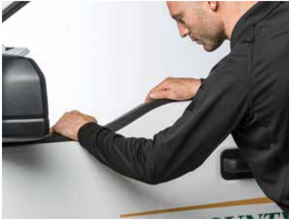
▲ Figure 13. Reinstalling outer window weatherstrip
