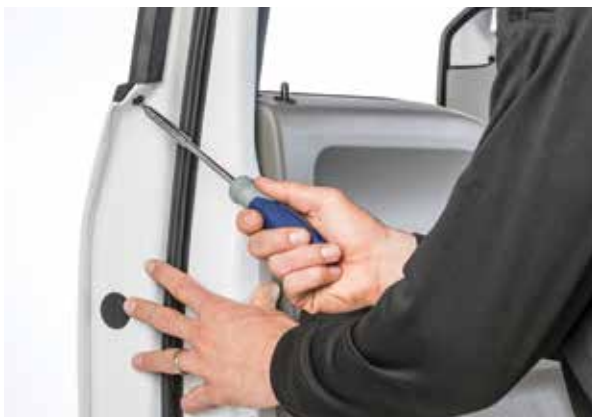
▲ Figure 6. Removing outer window weatherstrip screw
