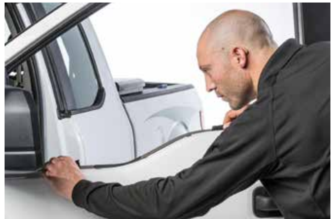
▲ Figure 11. Gripping and sliding the Ballistic Door Panel forward into place
