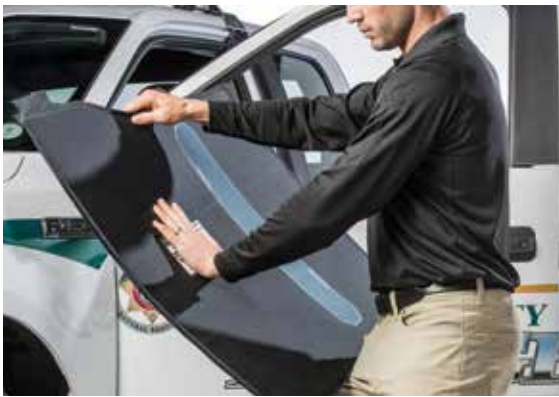
▲ Figure 9. Bending the Ballistic Door Panel to create a slight curve
