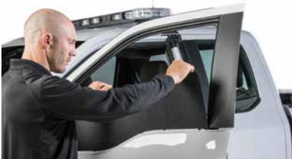
▲ Figure 10. Holding Ballistic Door Panel against window glass while leaning back
