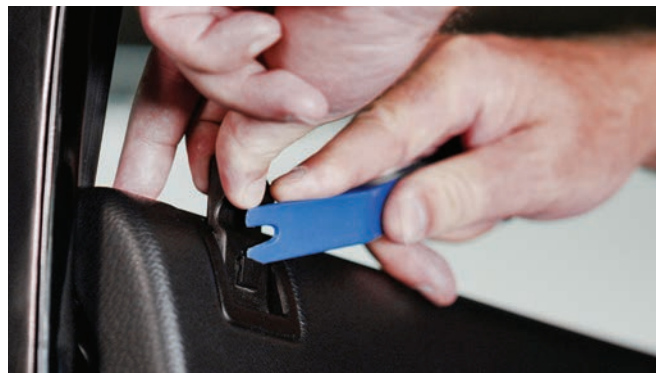
▲ Figure 5. Prying open the panel on the plastic lock knob
