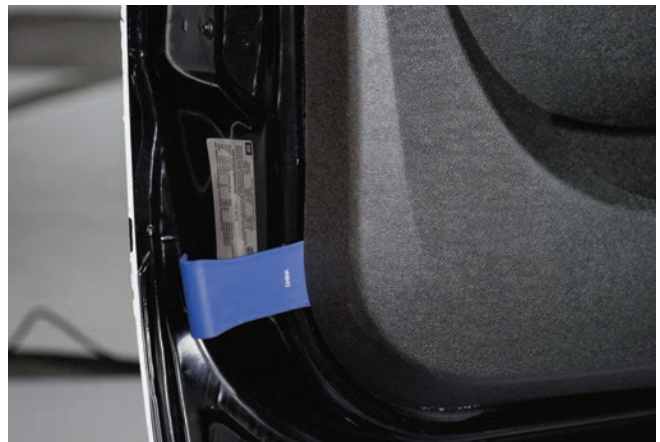
▲ Figure 8. Prying open the vehicle interior door panel
