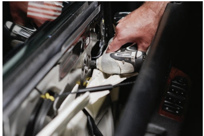
▲ Figure 10. Replacing the 10 mm factory-installed window regulator bolt with the supplied shorter 10 mm replacement bolt
