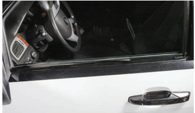
▲ Figure 15. Proper alignment of fold with window frame
