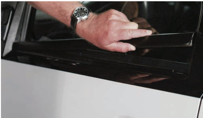
▲ Figure 11. Removing the outer window weatherstrip
