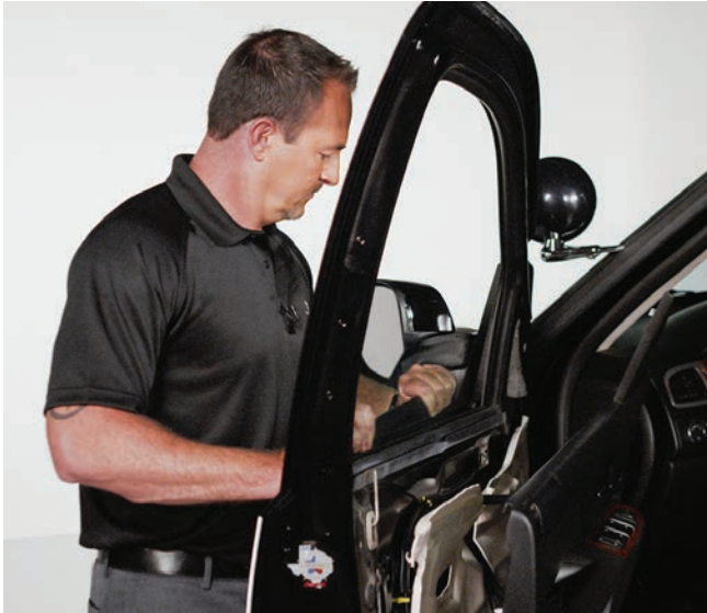
▲ Figure 13. Gripping ballistic door panel's top-edge nylon fold
